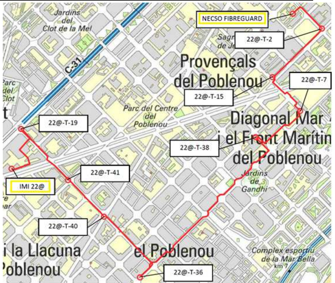
Figure 4: Fibre between IMI and Eurona with cabinets locations.
