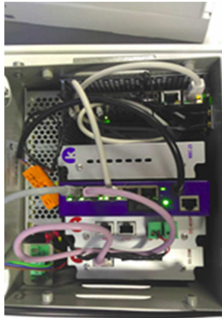
Figure 22 - Interior of the casing holding the SBC, battery, ethernet switch, power module, and an alarm module (top to bottom).
